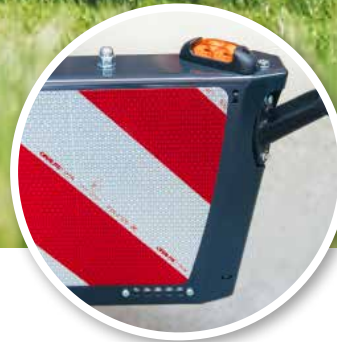
LED Streifen + Blinkerleuchten
